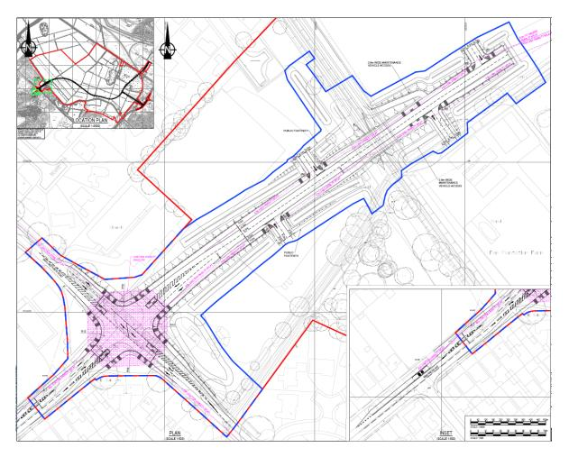
Originally proposed as a roundabout the applications took on board advice from the Highways Authority and have changed the site access to a signalled crossing. The highway capacity of both types of access were assessed, however the preference of a signal crossing has always been LCC's approach. A signalled crossing enables greater ease of movement for non-motorised modes of transport with footpath and cycleways proposed on all arms of the junction.
